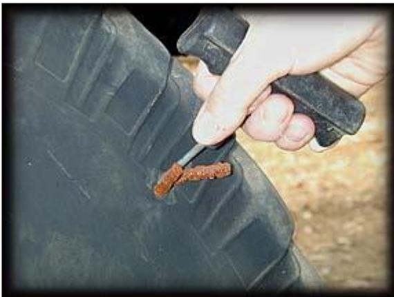
With about 1/2 inch of the material sticking out - jerk back the inserting tool with one swift move. The strip will stay in the hole. Most kits also include a vulcanizing solution which I found not much effective at all - therefore I do not use it for my repairs.
