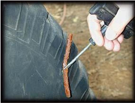
Simply place the 4 inch long strip into the cut out at the tip of the inserting tool (if necessary use the abrasive tool to enlarge hole) and push the assembly firmly into the hole. Click on image to view detail.
