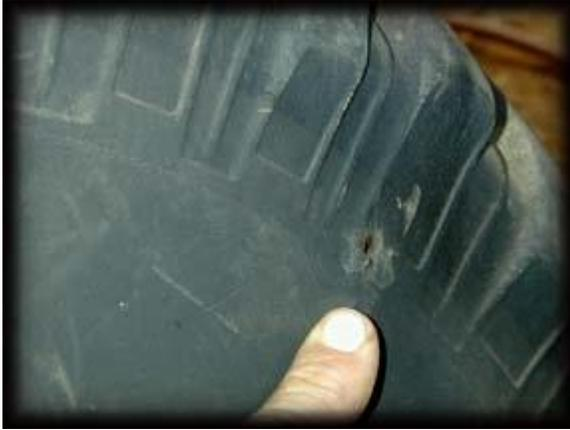
In off-road situations your tires will most likely develop a hole in the lower sidewall area. This is where steel belted tires are the softest and most vulnerable. The steel belted tread area is well protected from punctures.
