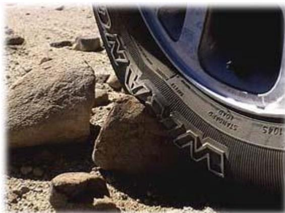
This image demonstrates the severe compression when a tire hits a rock off center.
